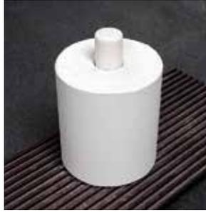
▶ Divest carefully using a hand-held microblaster or a WHIP Mix Xcavator automatic blasting unit to save time and labor.
